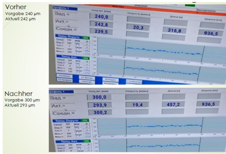
Figure 7: Representation of thickness distribution before and after changing process parameters (Task: Switch from 240 µm to 300 µm)
